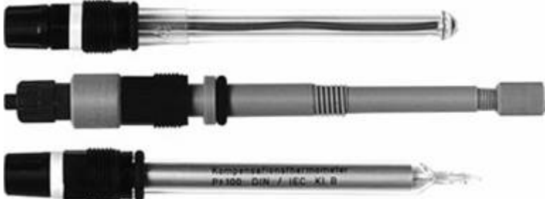
Fig.1: Several water sensors, length ~150 - 200 mm; Ø ~ 12 mm (source JUMO / Germany)
