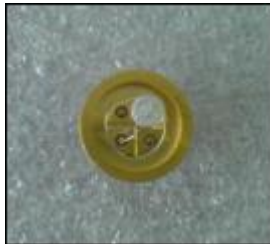
Fig. 5: Sensor for CO 2 detection with oxides sensitive layer (source ICPE-CA)
